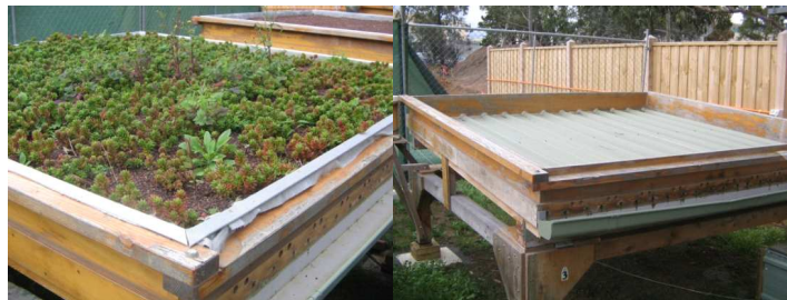
Figure 1. Two roof configurations monitored during the experiment: a vegetated (left) and an impervious roof (right).
